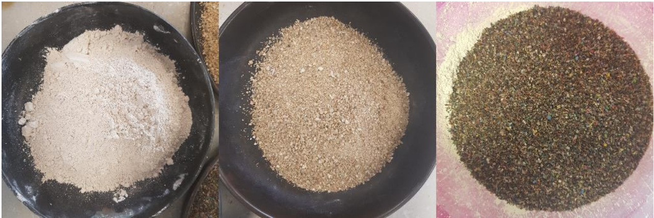
Figure 1. (Left) lime (Center) aggregate. (Right) plastic cable waste. Source: author's own creation
